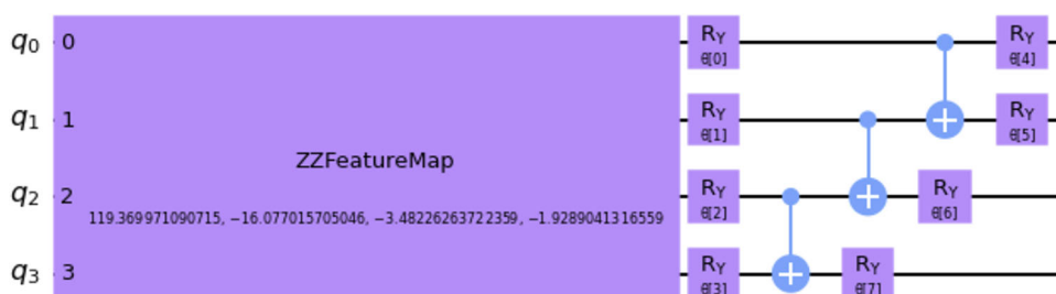
Fig. 6 Quantum random forest circuit. It consists of a feature map that encodes the input data, a layer of y rotation gates, CNOT gates between each qubit, and lastly a layer of z rotation gates
