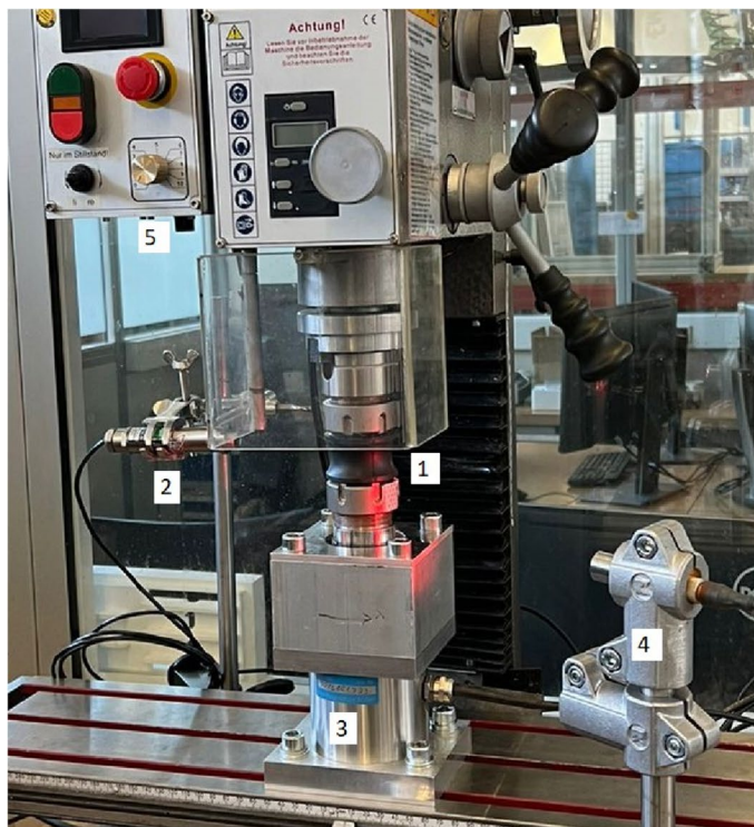
Fig. 1 Experimental set-up for rotating shear loading
