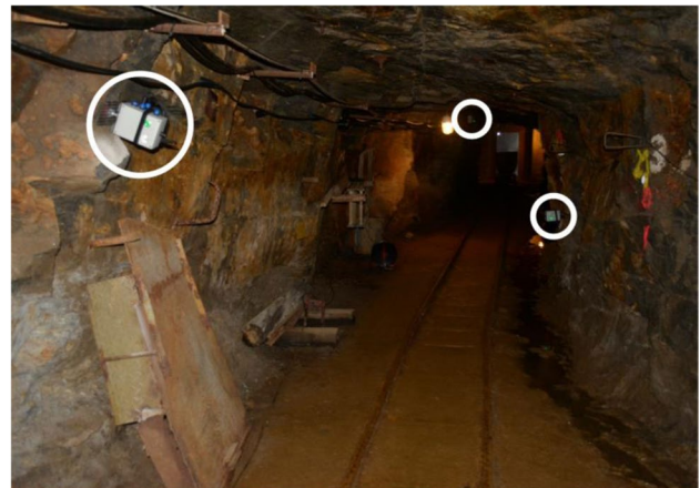
Fig. 19 The mine drift at Reiche Zeche with deployed anchors
