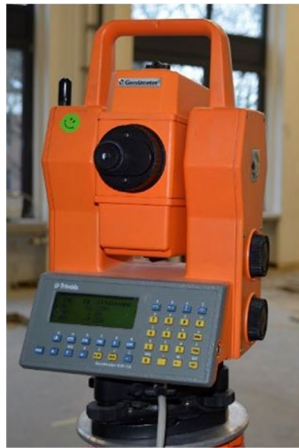
Fig. 16 Tachymeter used in the mine as a reference system
