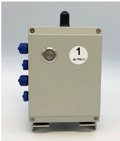
Fig. 12 The developed UWB module including the black outdoor antenna and the blue communication and power supply ports
