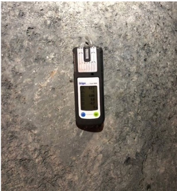
Fig. 7 A photo of gas monitor used to measure gases’ concentration during the field trial
