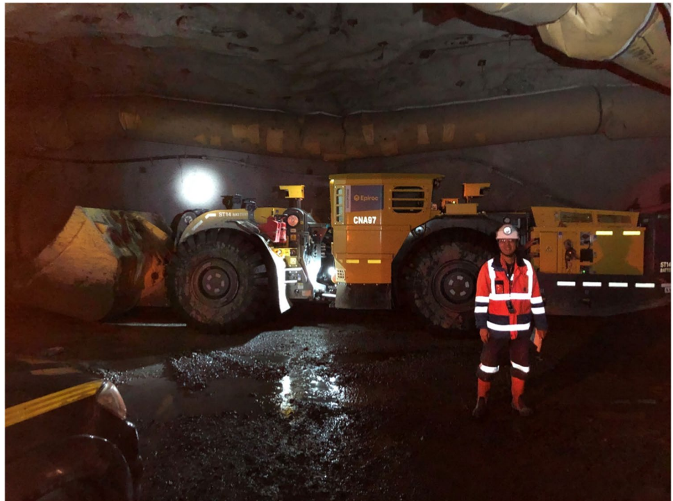
Fig. 5 ST14 Battery during the field trial in Kittilä mine
