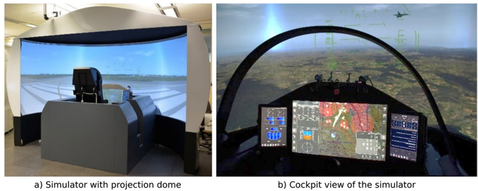
Fig. 8 Simulator setup, a view with the projection system, b view of the pilot
