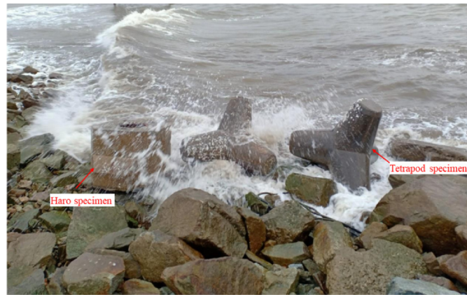
(a) In the real marine environment, Haro and Tetrapod specimens
