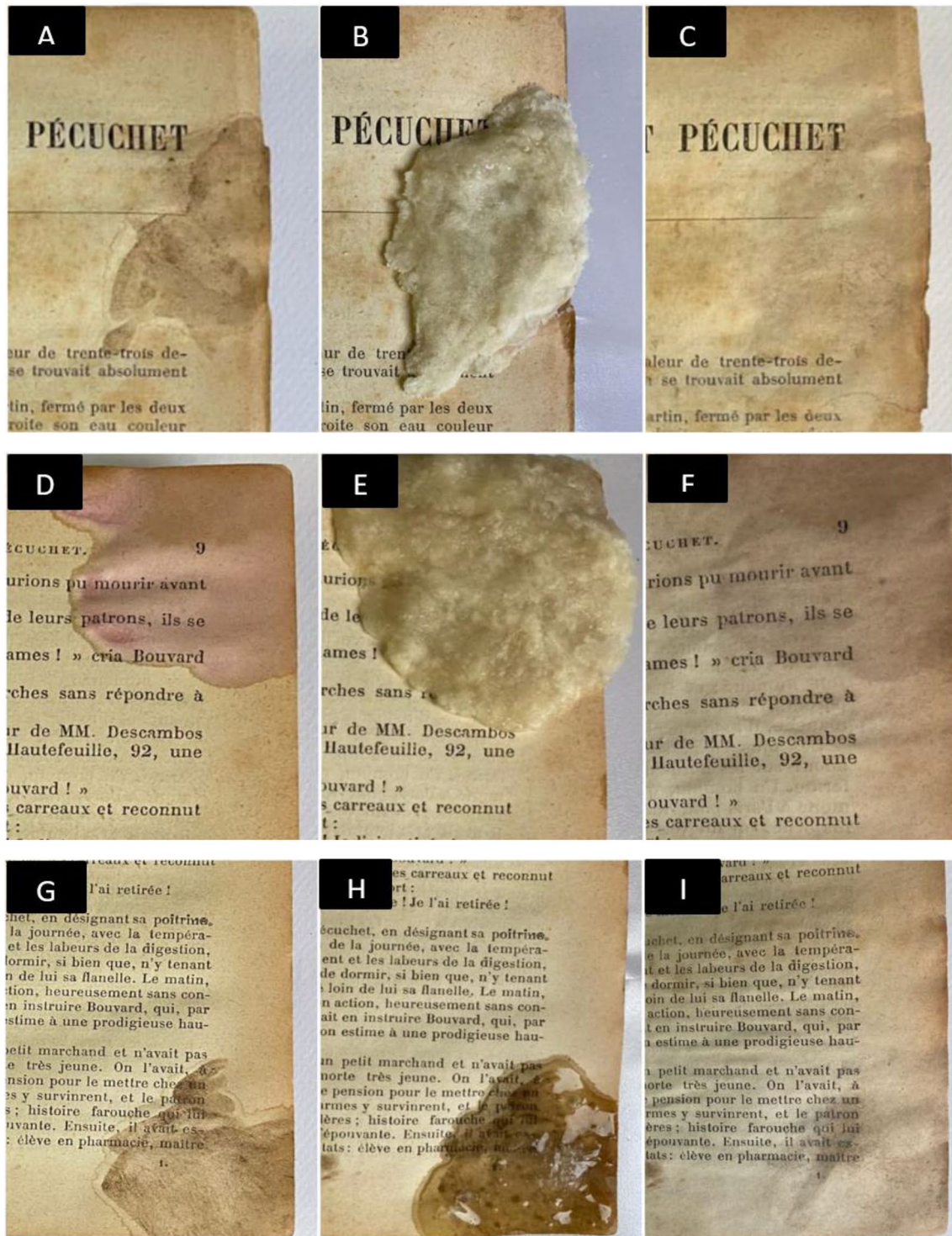
Fig. 3 Shows the cleaning of mud stain using compress of cellulose. The mud stain before cleaning (a), the mud stain during cleaning (b), the final result of cleaning of mud stain using cellulose compress (c), the pomegranate stain (d), the pomegranate stain during cleaning (b, e), the final result of cleaning furthermore as the cleaning of pomegranate stain using compress of gellan gum (f), the accumulation of mud particles on the surface (g), the role of gellan gum compress in removing mud stain (h), and the mud stain after cleaning, where the paper became more fragile (i)
