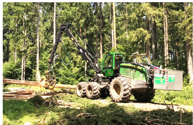
Fig. 2 John Deere 1470G harvester with installed PEMS at the rear
