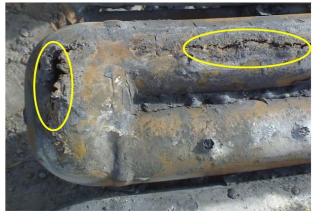
Fig. 12 Mechanical failure locations on WCPs hot-side [9]
