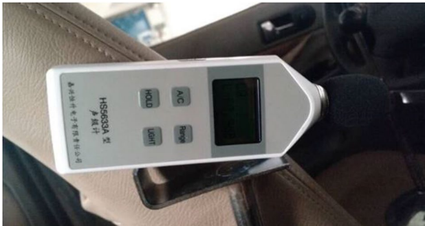
Fig. 4 Placement of sound level meter in car test
