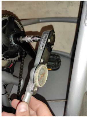
Fig. 12 Experimental set-up to estimate the double-chain transmission efficiency using a torque meter
