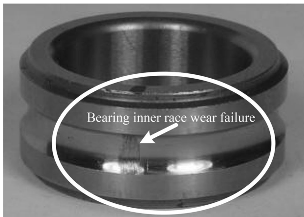
Fig. 5 Bearing inner race wear failure
