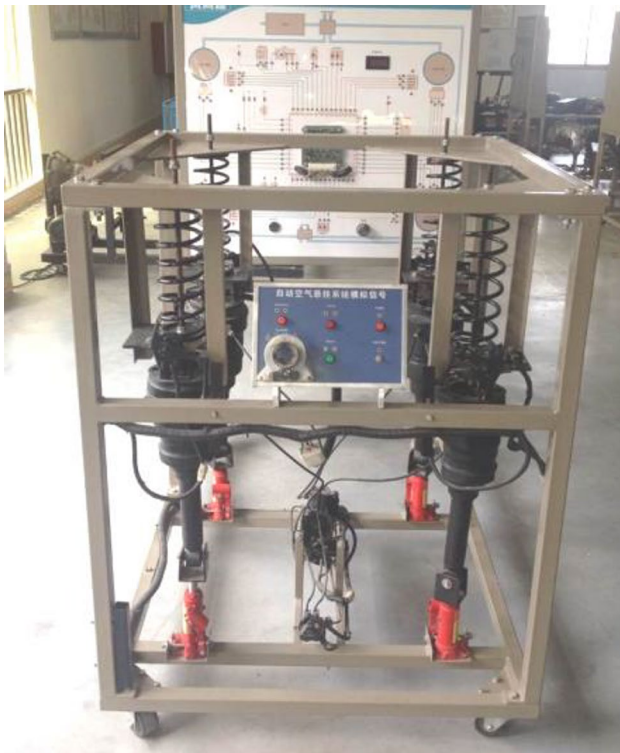
Fig. 1 Test Bench of Active Suspension System
