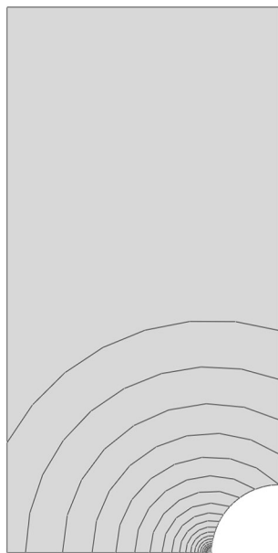
Fig. 4 Radial layers emanating from crack opening
