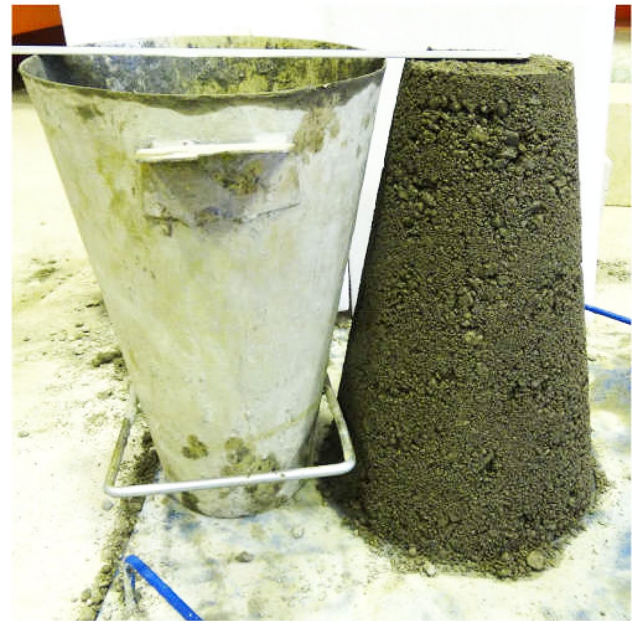
Fig. 7 The slump test of CSG mixture with 12.5% cement content and in the fresh state
