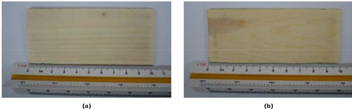
Fig. 6 Test specimens a Northeast China ash ( Fraxinus mandshurica ), b Korean pine ( Pinus Koraiensis )
