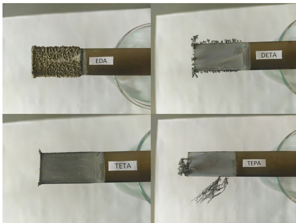
Fig. 1 Appearance of cathodic deposits of lead metal obtained from different polyamine electrolytes
