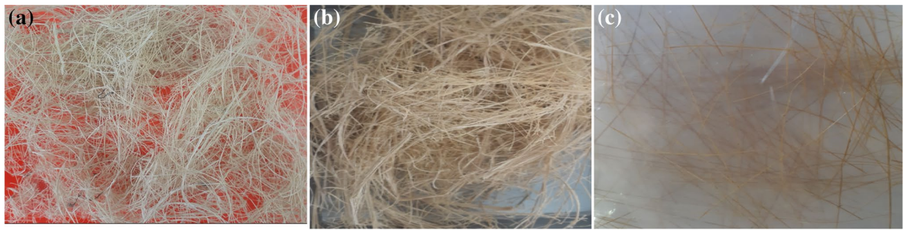
Fig. 2 Y.alpina bamboo fiber a Untreated b Treated c Treated fiber testing sample hold on a plastic holder
