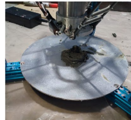
(b) Second test after adjusting the slicing parameters (printing speed 26 mm/s)
