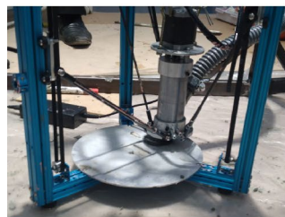
(a) First test (air pressure 90 PSI and printing speed 28 mm/s)
