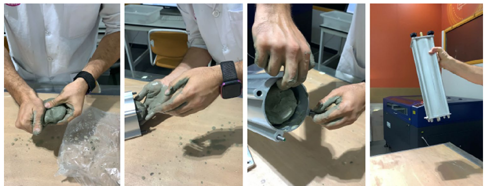
Fig. 2 Preparation and loaded clay into a container
