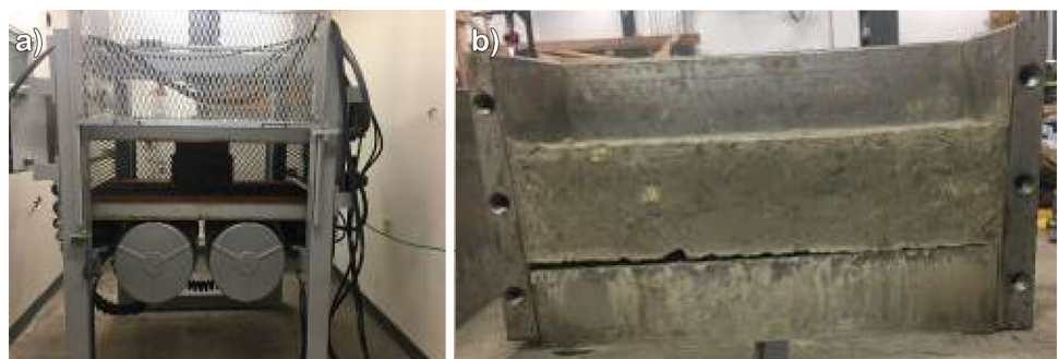
Fig. 1 a, b. Dynamic high-pressure compaction system (a), high-pressure compacted Portland cement particle fiber mixed block (b)
