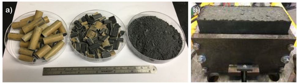
Fig. 4 a High voltage hybrid FCP admixtures that were processed into chips (middle) and a powder ( \sim 52.85 \mu\text{m} ) (far right), and then b mixed with Portland cement and water and high-pressure compacted into a solid rectangular brick-shaped material
