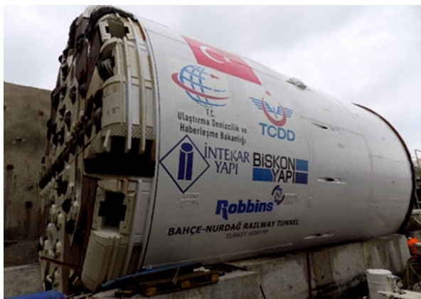
Fig. 5 The TBM used in Bahçe–Nurdag tunnel
