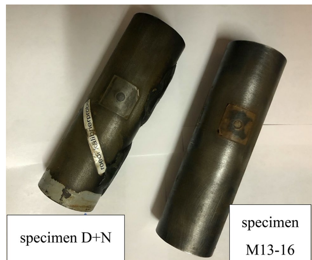
Fig. 3 Shot peened specimen D+N and M13-16. The measuring direction was along the bar
