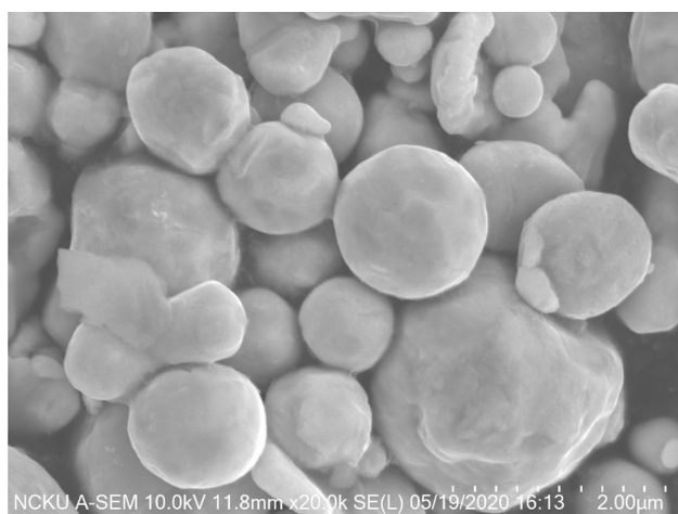
Fig. 1 SEM morphology of silver powders
