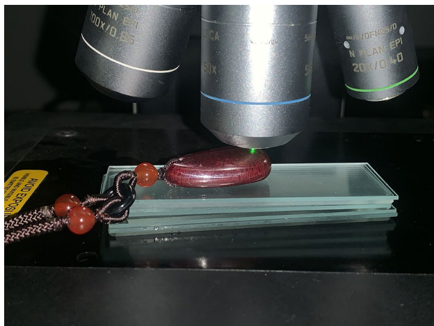
Fig. 6 Micro-Raman experiment scene for the raw mineral sample
