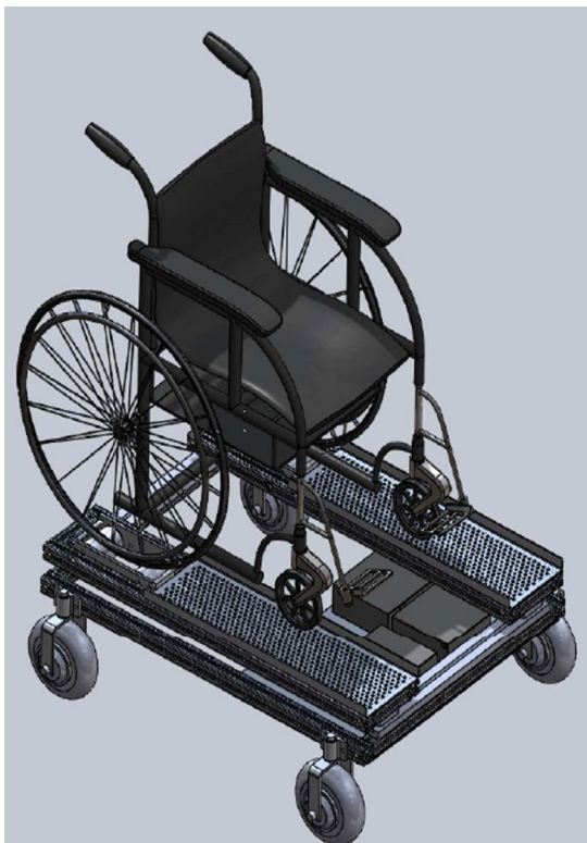
Fig. 1 A basic illustration of the carrier platform with the wheelchair mounted on it
