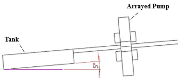
Fig. 20 The angle of the reservoir and pump with the horizon
