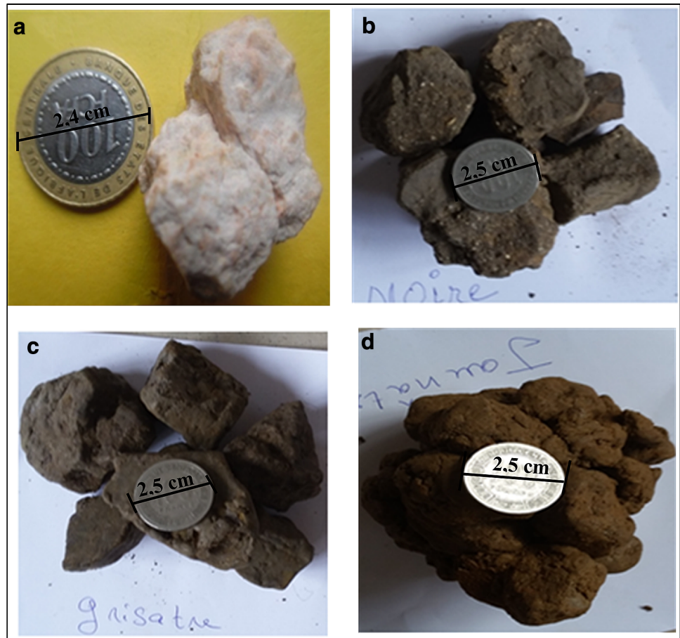
Fig. 1 Raw material showing: a Feldspar crystal, b Black clay, c Gray clay, d yellow clay
