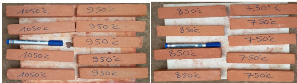
Fig. 5 Fired bricks at different temperatures
