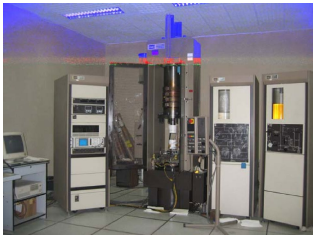
Fig. 5 Rock testing system
