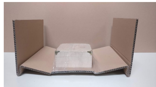
Fig. 3 Insufficient panel stiffness
