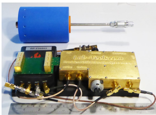
Fig. 1 A highly compact lab-tools Mk3 time-domain NMR spectrometer and light-weight mandhalas NMR magnet, both designed especially for low-field material science NMR relaxation and NMR cryoporometry pore size measurements, in the lab and in the field
