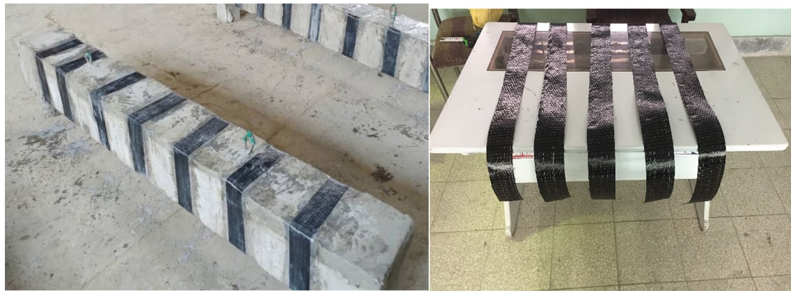
Fig. 4 FRP strips preparation
