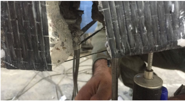
Fig. 12 Rebar failure pattern in SBDRS
