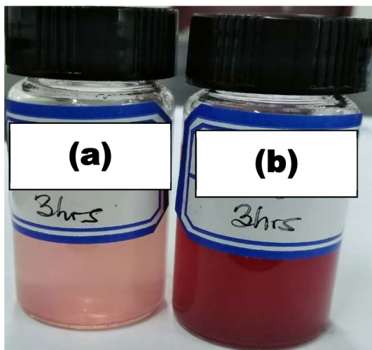
Fig. 2 Colour of a 20 mL Et-ACPE/100 mL H 2 O and b 20 mL ACPE/100 mL AgNO 3 (Et-AgNPs) after three hours of formation of NPs
