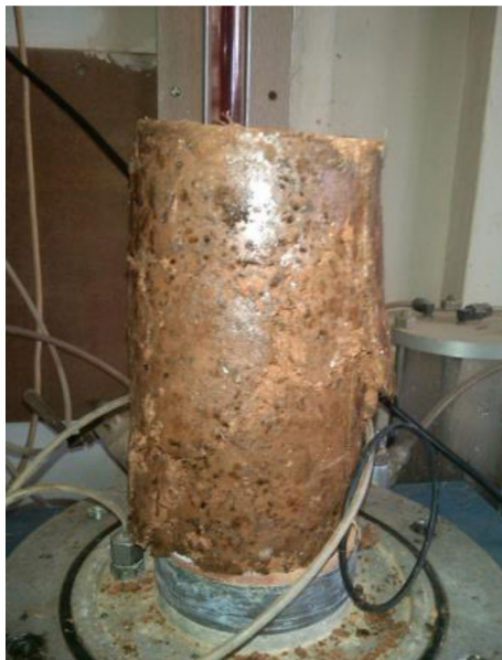
Fig. 13 Failure by bulging for 0.2% FC
