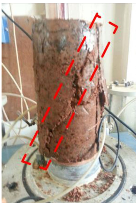
Fig. 14 Failure by shearing for 0.6% FC
