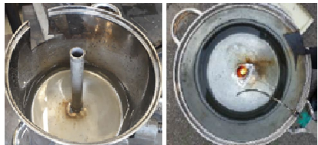
Fig. 2 The pot to be put on the plate or ring and which was perforated by a tube in its center, to periodically inject the pellets in the combustion zone
