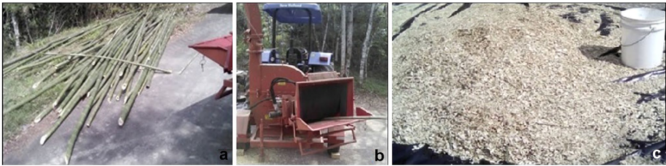
Fig. 1 Bamboo chip production process. a Bamboo stems (thirty units); b Forest Chipper coupled to the hydraulic system of a farm tractor used to cut bamboo stems into chips; c total volume of chips produced
