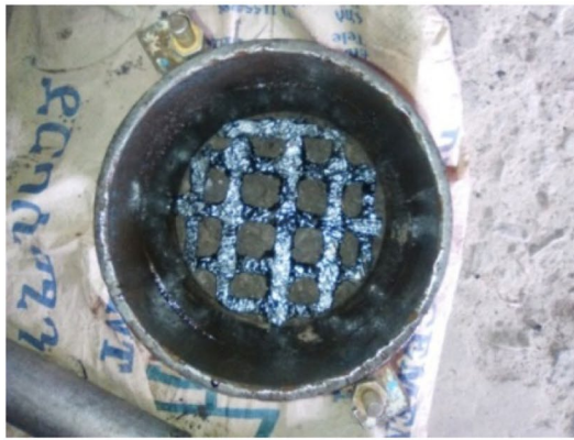
Fig. 5 Placement of Polypropylene (PP) and High Density Polyethylene (HDPE) type of geogrid material inside CBR mold 35 mm below Plunger bottom
