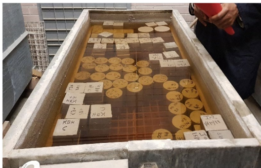
Fig. 4 Concrete cubes and cylinder specimen in a curing tank
