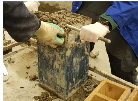
Fig. 8 Levelling the top of the mould
