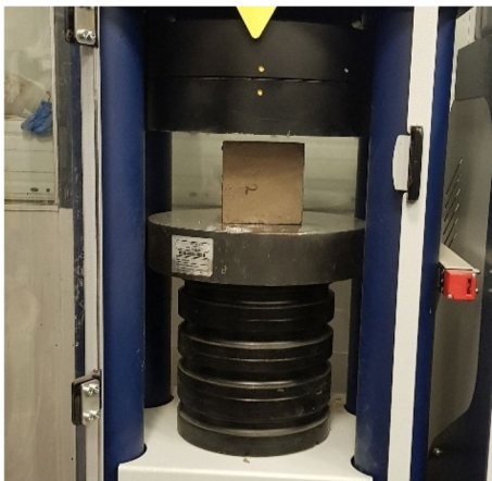
Fig. 10 Applying vertical force to cube specimen
