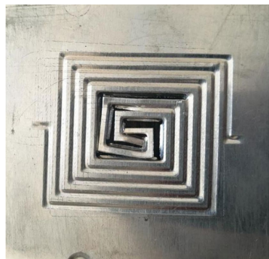
Fig. 5 A ruptured produced sample due to the applied excessive press forces; polyurethane pad, punch speed of 8 mm/s, press force of 50 ton
