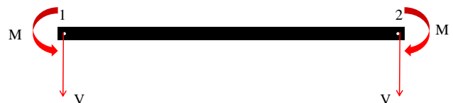
Fig. 3 Loaded beam element
