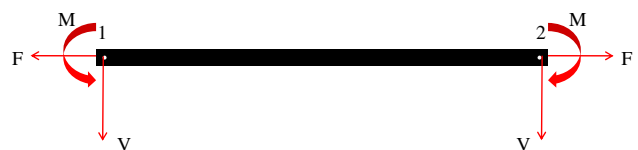
Fig. 4 Loaded frame element
