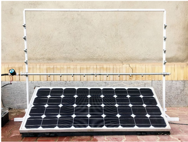
Fig. 3 PV module under the water spray cooling with its specific experimental setup
