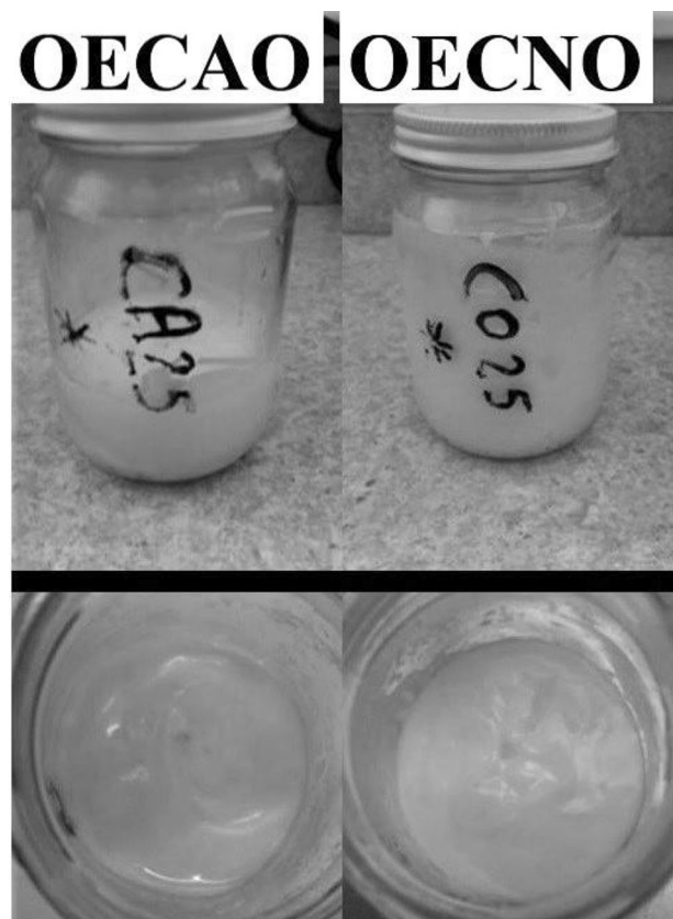
Fig. 1 Macroscopic appearance of organogel-emulsions canola oil (OECAO and coconut oil OECNO) at 28 days
