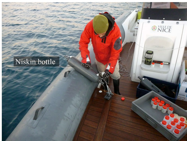
Fig. 4 Sampling using a Niskin bottle
