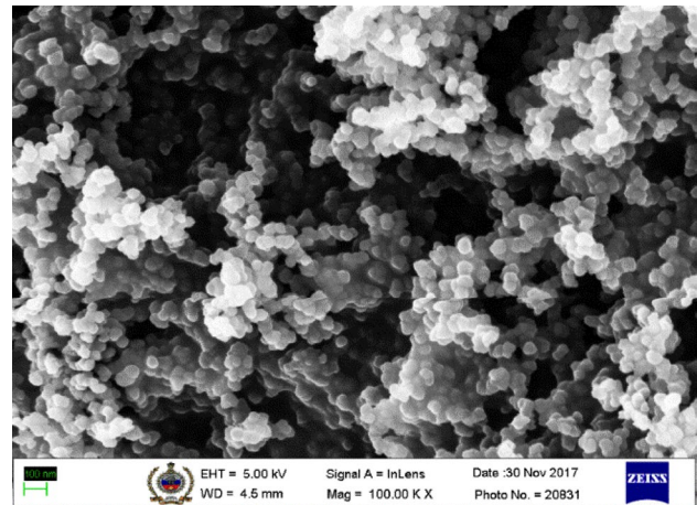
Fig. 3 FE-SEM image of carbon soot particles generated from waste plastic
