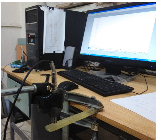
Fig. 9 The modal analysis test of the FGM beams
