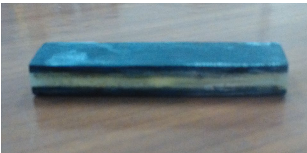
Fig. 7 Three-layer FGM beam with pure epoxy at mid-plane and 3 wt % MWCNT/epoxy at the upper and lower layers
