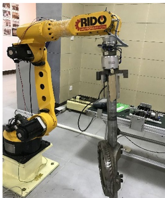
Fig. 11 Modal test in progress
