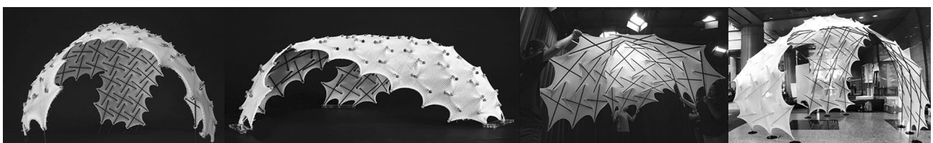
Fig. 9 Design variations of the knit tensegrity shell, expressed in 1:10 scale models and full-scale prototypes
