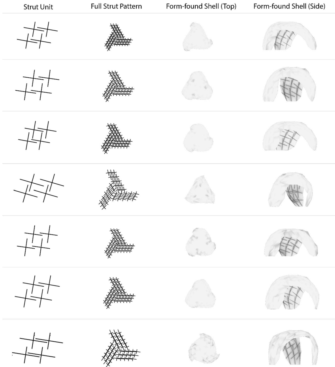
Fig. 3 Illustrative catalog of various digital shell geometries based on different strut tessellation patterning
