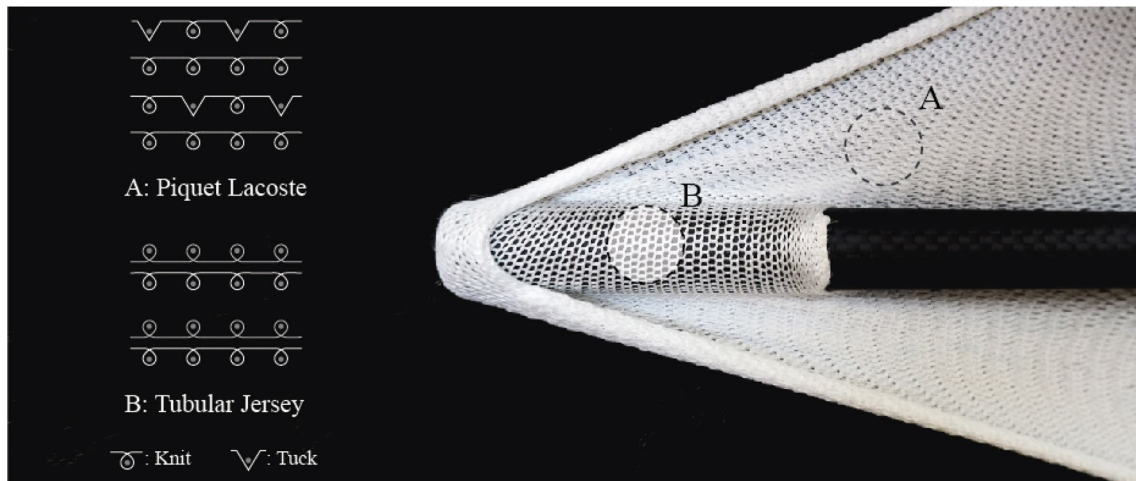
Fig. 7 Left—Knit notation for piquet lacoste (main body) and tubular single jersey (pockets); Right—Pocket with carbon fiber strut end inserted inside
