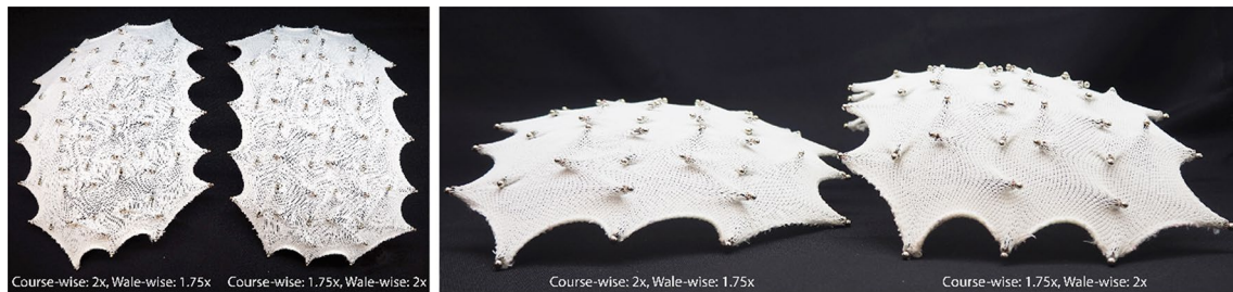
Fig. 5 Comparison between two models with the same strut pattern but different amounts of stretching. Left—Top view of membrane stretched 2× along the course-wise axis and 1.75× along the wale-wise axis; Second from left—Top view of membrane stretched
