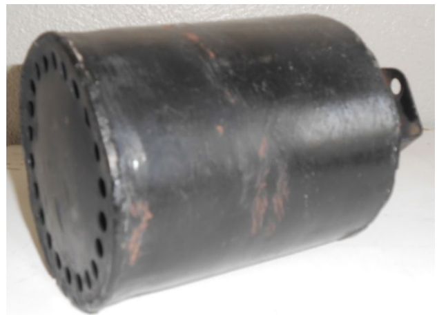
Fig. 4 Prototype of new developed muffler
