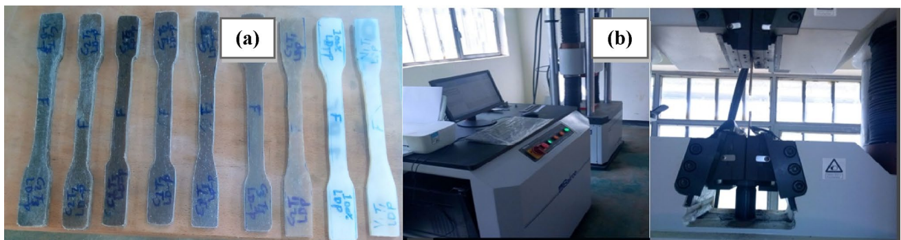
Fig. 6 a Specimen samples after cutting, b Specimens under tensile strength test
