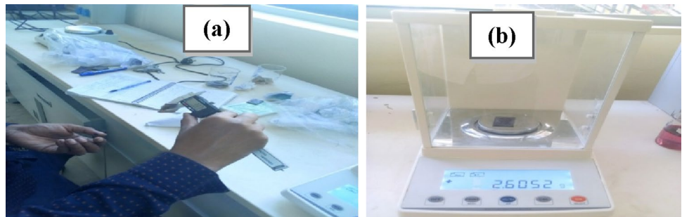
Fig. 10 a Measuring Specimen in digital caliper, b Specimen at balance weight
