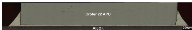
Fig. 7 Digital microscope overview of the complete RAB joint area ( T_b = 1000\text{ }^\circ\text{C} , t_d = 5\text{ min} )
