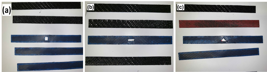
Fig. 1 Prepreg strips of the specimens have a square cut-out, b rectangular cut-out, c triangular cut-out defect
