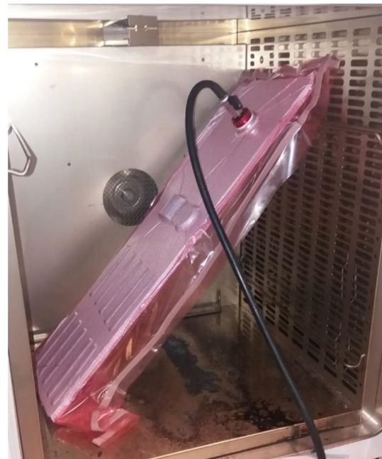
Fig. 3 Specimens curing in a vacuum bag and undergo curing cycle in an oven
